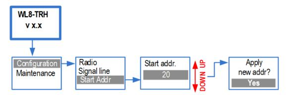
Each wireless device will also have its own address in the main control panel. The numbering will begin with the starting address of the translator. For example, if the starting address is "1", the following wireless devices that are added to the system will be given address "2", "3", "4", "5" and so on. If another starting address is specified, for example "34", the wireless devices will be automatically readdressed with "35", "36", "37", "38" and so on.
